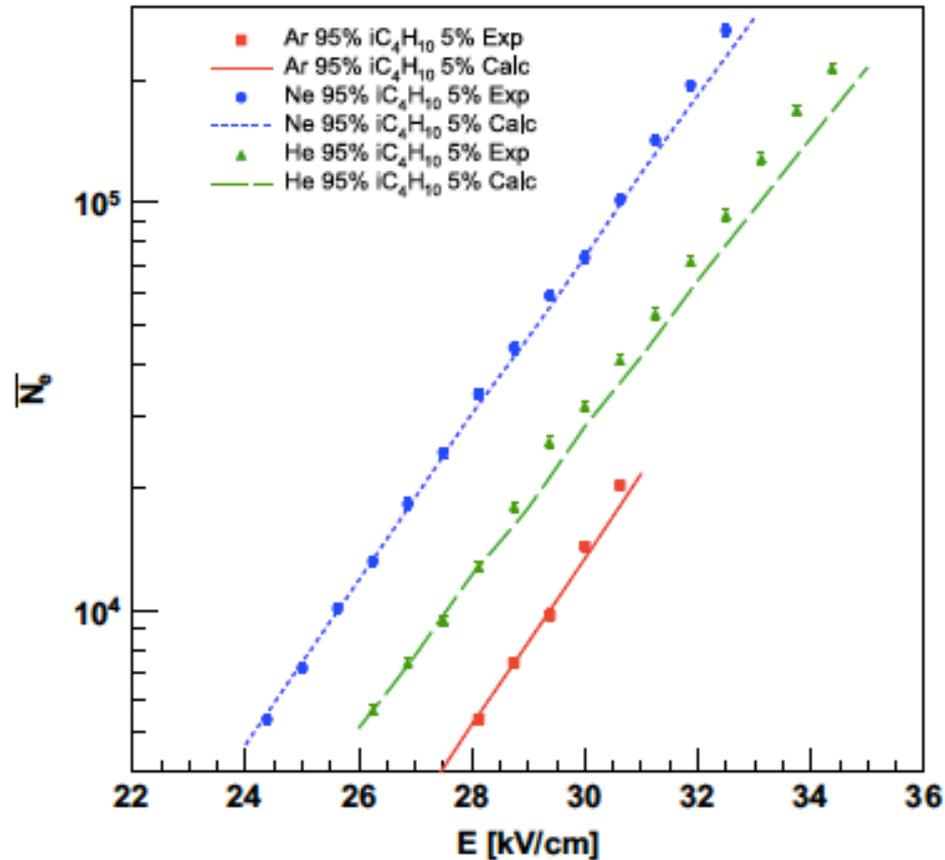
Fig. 6. Experimental mean gains  $\overline{N_e}$  as a function of the amplification field  $E$  compared with the Monte-Carlo simulations for the argon, neon and helium gas mixtures.
