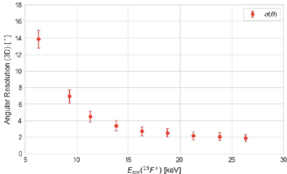
**Figure 8.** MIMAC angular resolution as a function of  $^{19}\text{F}$  ion kinetic energy. At lower energies, the ion tracks are shorter and have more straggling resulting in worse angular resolution and bigger error bars. The angular resolution is better than  $20^\circ$  down to a kinetic energy of 6.3 keV, and is below  $10^\circ$  for a kinetic energy of 9.3 keV. Error bars are derived from the pixel strips pitch and reconstructed track length as described in the text.
