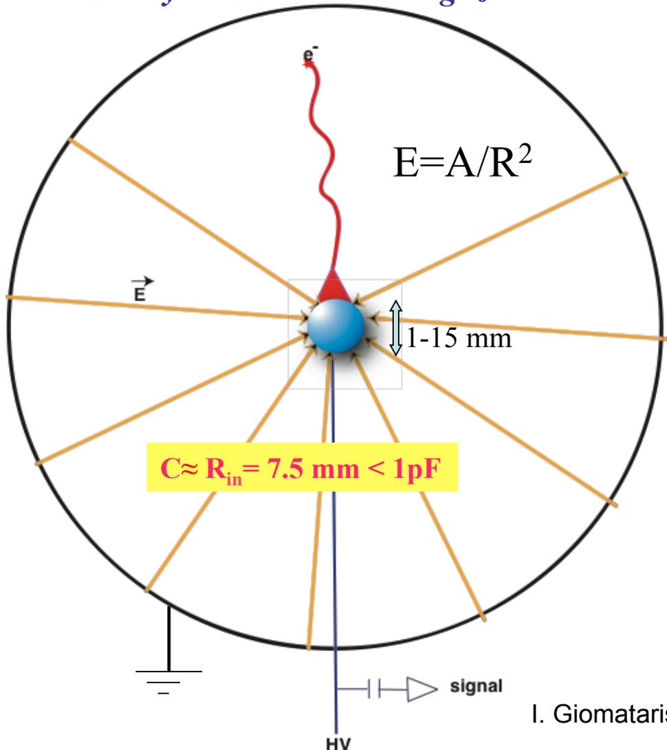
A Novel large-volume Spherical Detector with Proportional Amplification read-out, I. Giomataris *et al.*, JINST 3:P09007,2008
