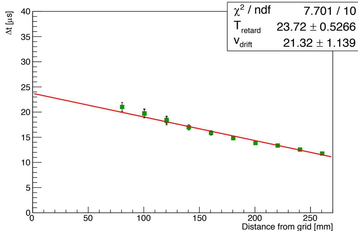
**Figure 4.** Measure of the time differences (TAC) between the grid signal and the delayed cathode signal in the “START Grid” configuration, as a function of the distance of the  $\alpha$  source from the anode (green points) ; error bars correspond to the standard deviation of the mean. A linear fit of these points is superimposed in red and provides the values of the drift velocity and the additional delay.
