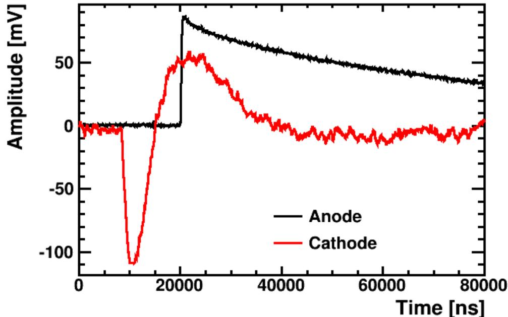
Measurement in a MIMAC chamber of an alpha passing through the active volume parallel to the cathode at 10 cm distance.
