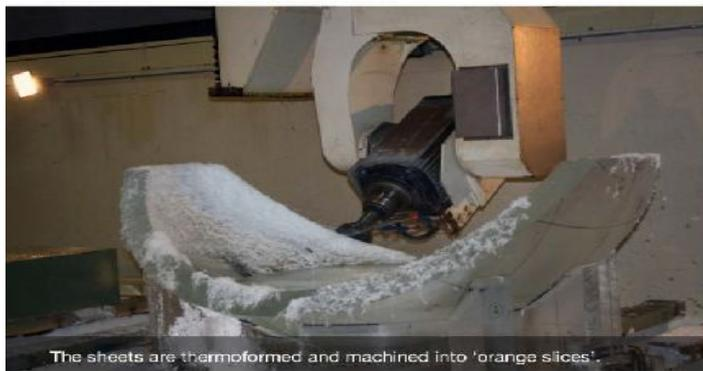
The sheets are thermoformed and machined into 'orange slices'.
