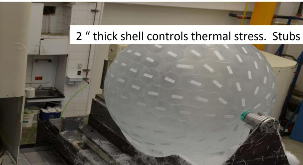
2" thick shell controls thermal stress. Stubs move bond to low stress regions.
