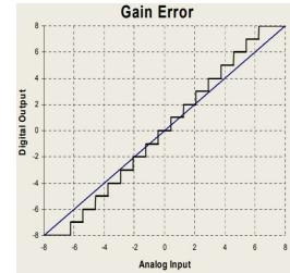
Slope issue, can be corrected using a second point reference voltage
