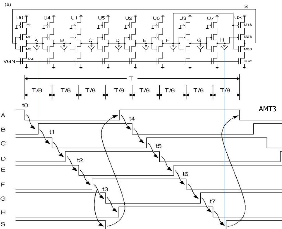
Fig. 2 (a) Asymmetric ring oscillator, (b) extracted timing signal.
