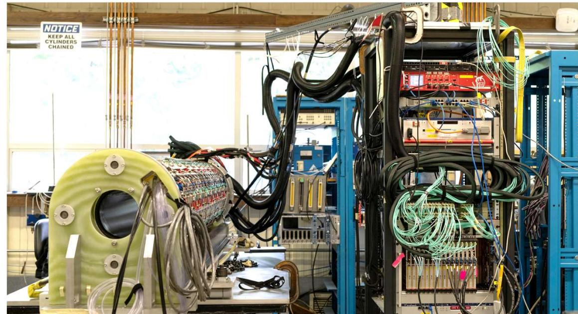
Large portion of the frontend electronics including the waveform digitizers reside on the detector (256 ASICs)
