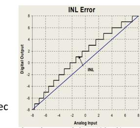
Cannot be corrected, due to ADC architecture
