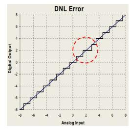
Cannot be corrected, due to ADC architecture
