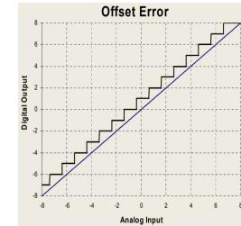
Can be corrected using a reference voltage
