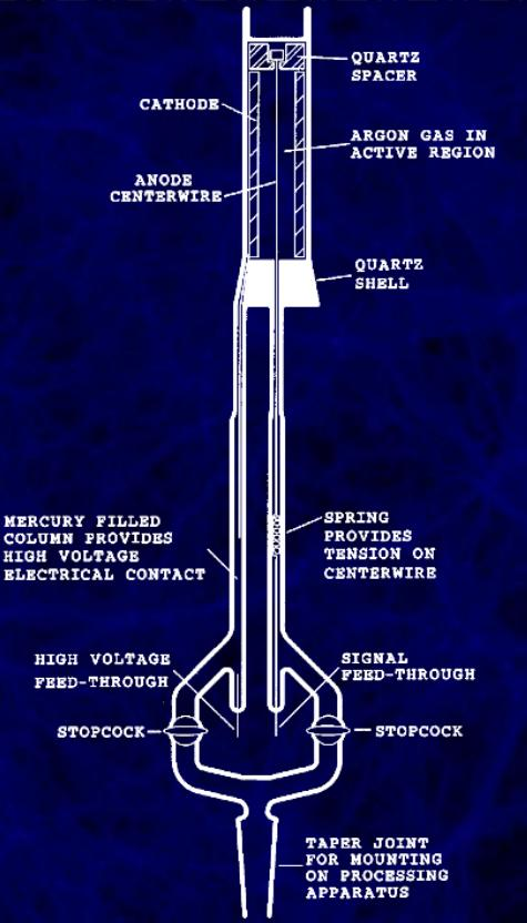
FIG. 7.—Proportional counter geometry. Sketch of the miniature proportional counters used to observe  $^{37}\text{Ar}$  decays. Counters typically have an overall length of 20 cm, with an active region 30 mm long and 4.5 mm in diameter.
